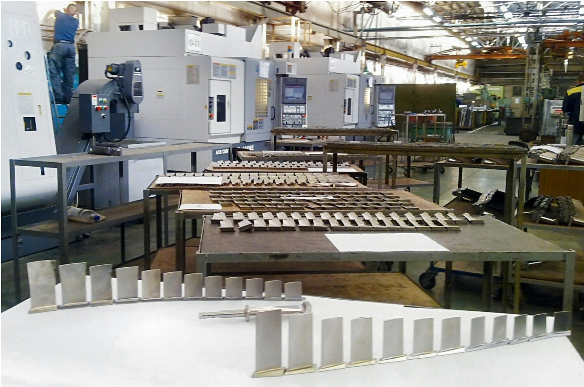
Working and guide compressor blades of 1st-12th stages of gas turbine GTU - 8 (8 Mw)
